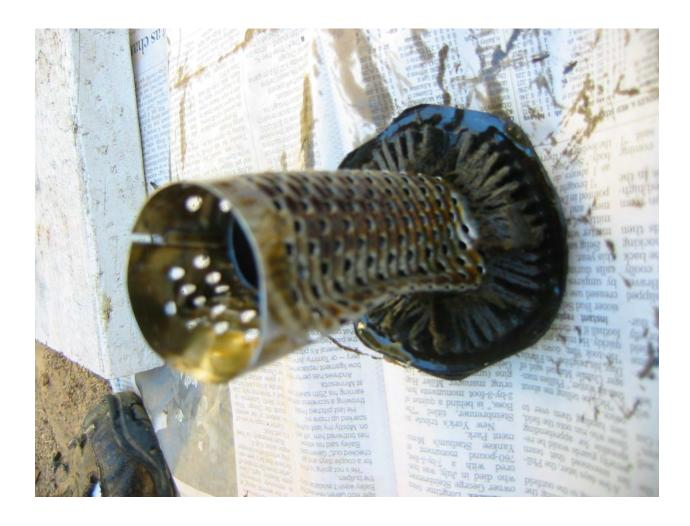
There should be an annular space between the inner standpipe and the outer perforated tube:
