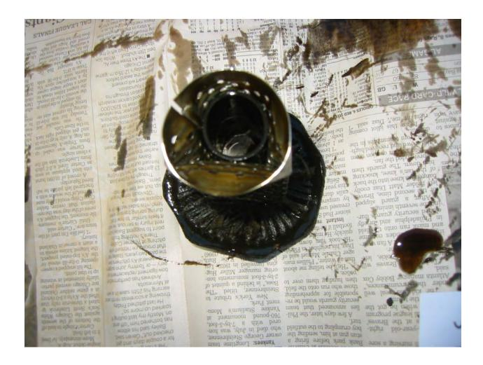
The perforated tube could not stand up to the force created by the oil flowing inward through the paper pleats:
