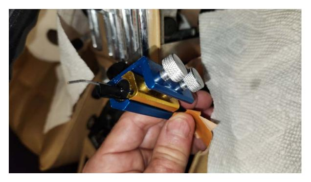
6) Put paper towels around the interior to catch any overspray or drips. Insert the red lubricant can straw into the lube tool lubricant hole on the side of the tool and press the lubricant can valve to force lubricant into the cable. \*\*\* this can be a little messy if the tool is not tightly clamped to the control rod sheath.
