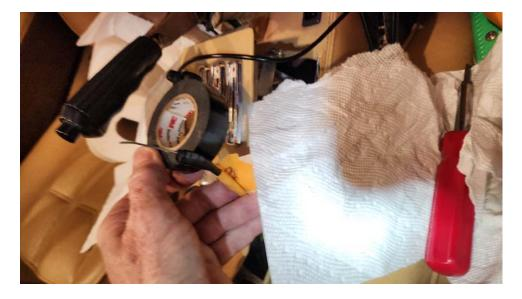
3) Take a small piece of electrical tape and put it around the control rod to increase the lube tool seal on the control rod which will stick out the end of the lube tool
