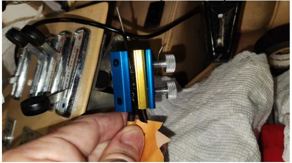
5) Tighten the knurled knobs on the lube tool down evenly as tight as you possibly can
