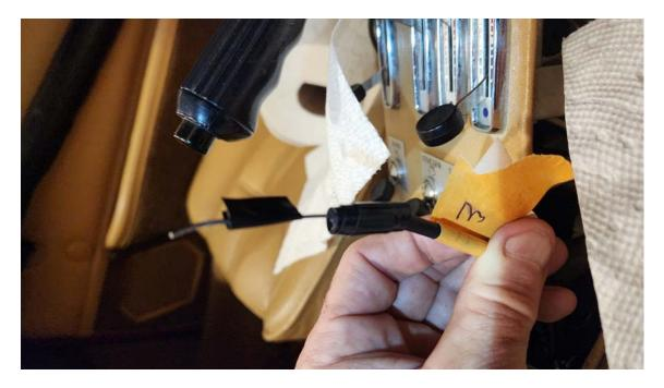
4) Place the lube tool onto the control rod sheath with the control rod sticking out the end of the tool and the small piece of electrical tape approximately 1/8 of an inch into the tool, be careful not to cover the lubricant inlet hole with the small piece of electrical tape on the wire
